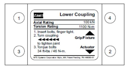
Installing an Axial-Torsional Adapter
