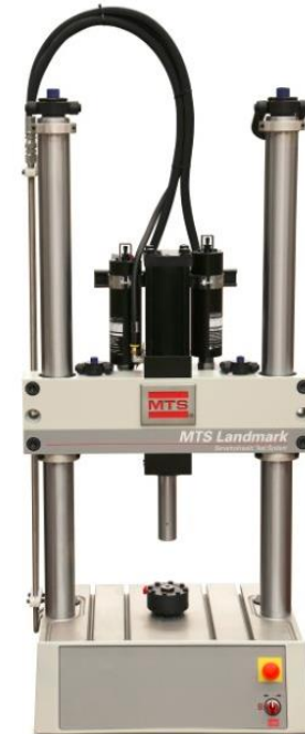
Load Frame - Position Transducer - Force Transducer - Servo valve - Hydraulic Service Manifold
