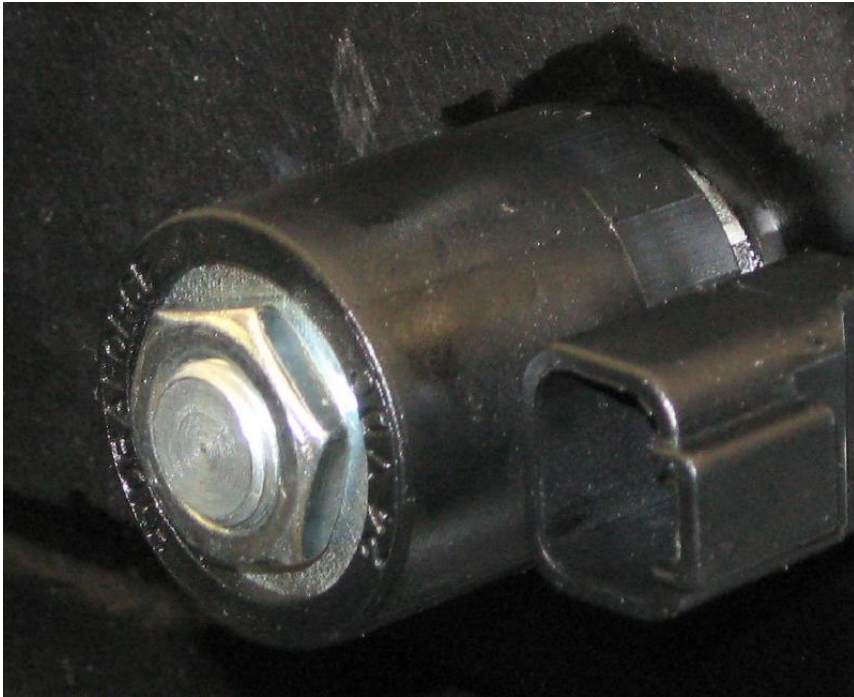
Low flow cartridge valve coil uses connector Deutsch DT04-2P
