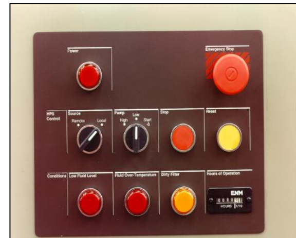
Emergency Stop Button located in photo, top right red round button. This is on a typical Hydraulic Power Unit.
