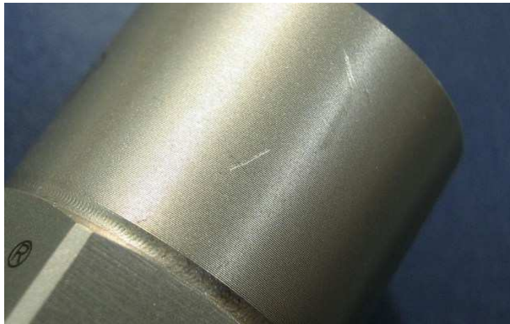
Figure 12 Unacceptable Scratches on Part Example
