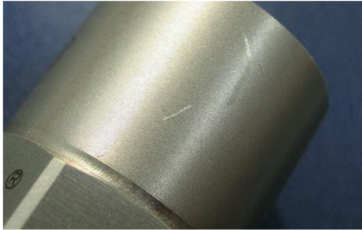
Figure 12 Unacceptable Scratches on Part Example
